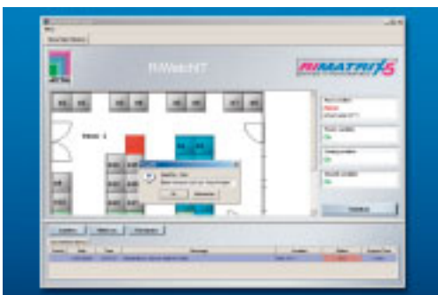
RiWatchIT allows you to monitor the on-going operation of a data centre.
