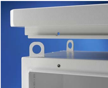
Eyebolts on the inner roof, concealed by the rain canopy, for crane transportation of the fully fitted unit.
